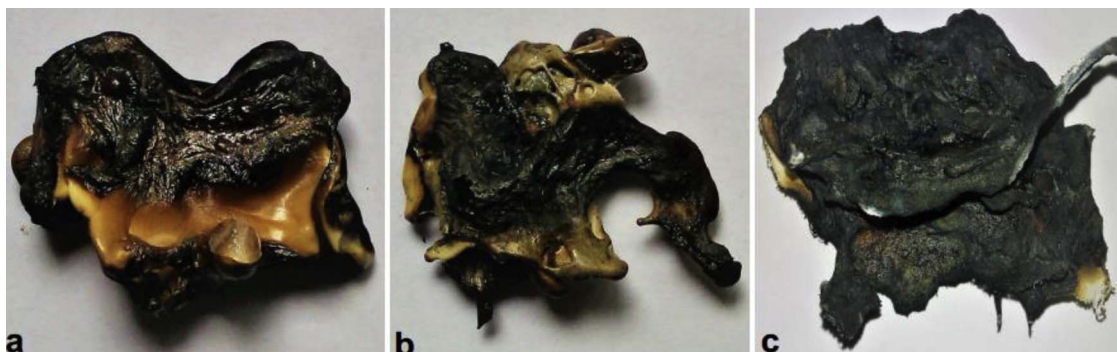
Fig. 4. Digital images of PA6.6 fabric samples (a. PA6.6 Control, b. PA6.6-PCS-4W, and c. PA6.6-PCS-4W-SG) after burning.
