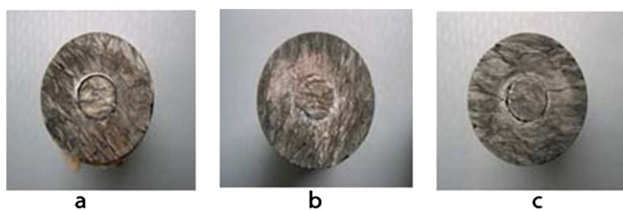
Figure 7. Specimens after arc jet evaluation. a) ACPR, b) ACPR 3 and c) ACPR 10. This figure is available in colour online at wileyonlinelibrary.com/journal/pat
